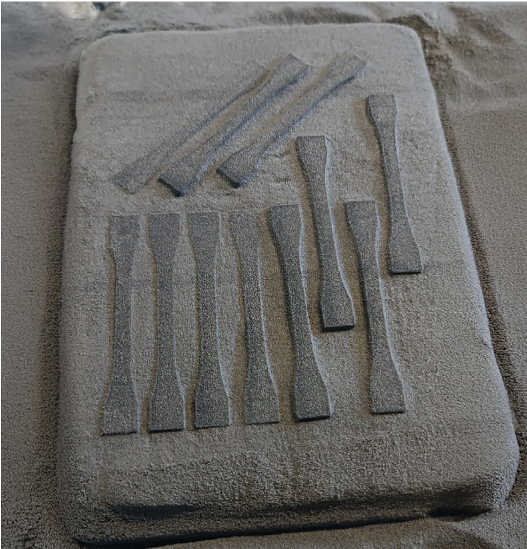
Depowdering of parts printed out of spherical polyolefin powder, Alpha Powders
